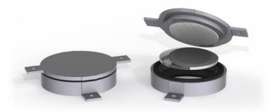
machined as a spherical surface to realize the hinge for rotation around every axis; the rotational surface is obtained coupling a curved sheet of PTFE and a spherical low roughness sliding surface (according with EN1337-2 code) to minimize friction and maximizing PTFE service life. In this "two plates configuration", the horizontal load is transmitted through the spherical surface to the base plate, according to design codes (as EN1337-7).
