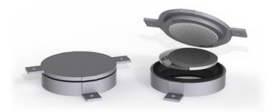
machined as a spherical surface to realize the hinge for rotation around every axis; the rotational surface is obtained coupling a curved sheet of AgomGlide® and a spherical low roughness sliding surface (according with EN1337-2 code) to minimize friction and maximizing AgomGlide® service life. In this "two plates configuration", the horizontal load is transmitted through the spherical surface to the base plate, according to design codes (as EN1337-7).
