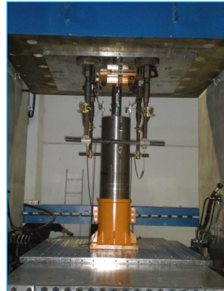
STU device tested at the EUCENTRE independent test laboratory
