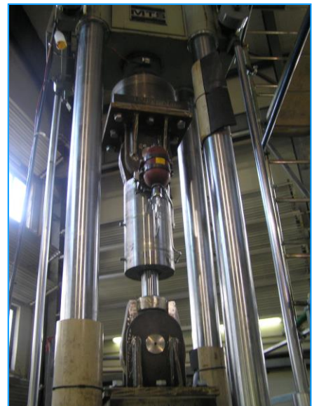
VD damper device tested at the Politecnico di Milano independent test laboratory
