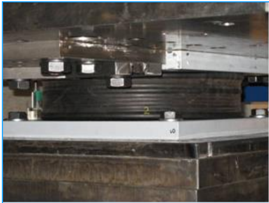
Isolator subjected to a very severe vertical load test with applied load 3 times the design value
