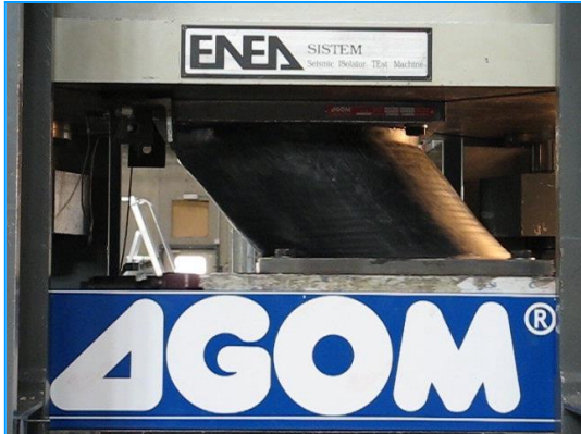
Isolators dynamic shear-compression tests at independent test laboratory
