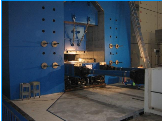
Isolators dynamic shear-compression tests at independent test laboratory
